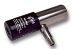
• Pirani gauges simply measure resistance in a (usually platinum) wire exposed to vacuum. Current heats the wire up (resistance goes up), collisions with ambient gas cool the wire down (resistance goes down).
