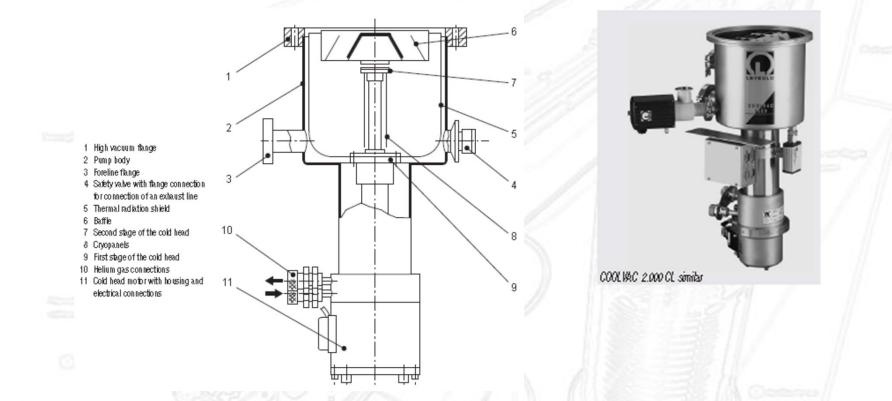
• These pumps work by condensing gas onto a surface that is cooled to  $I\!N_2$  temperatures.
