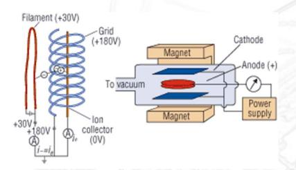
• Electrons generated from a heated filament ionize gas, which is drawn to a negatively charged filament inducing a measurable current. Electrons are discharged on a positively charged grid.
